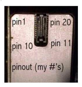
Hold the device so that the connector is upward. The pinouts are numbered here as if you were looking at a chip, that is starting at the upper left and proceeding down the left side and up the right side:
