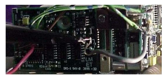
Now that the power board is exposed, solder a stub on the coax board point; that's where the frequency output is. It's a sine wave, probably will not drive very much. Just to the left of this point is a comparator that will give a pulse out at the frequency of the output. This comparator drives the divider chain to get a 1 second pulse.
